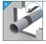
Remove the protective film on the back 1) and wrap the required number of layers of Multiwrap around the service penetration.
