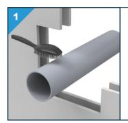
Make sure that the service penetration and the gap are free from dust, dirt and grease.
